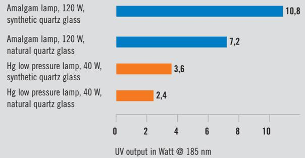
The UV power comparison relates to lamps with the same illuminated length of 800 mm and the same tube diameter of 15 mm
